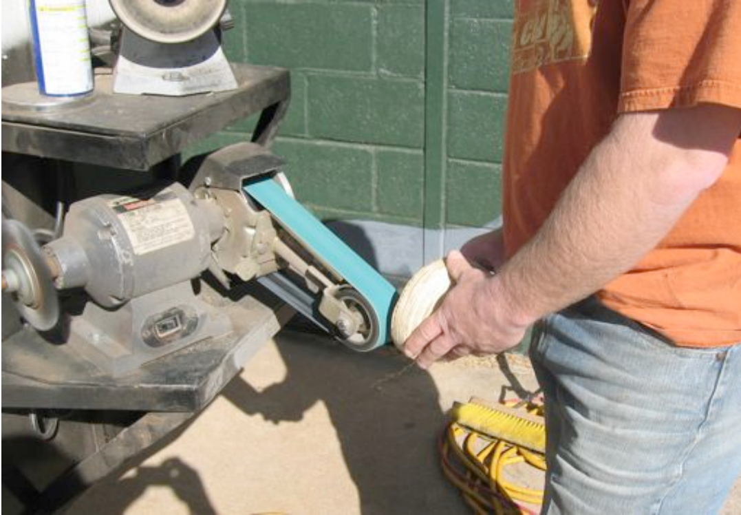
Fig. 4. The combination belt sander/grinder is a very useful tool employed by many farriers. The belt sander makes fast work of applying breakover in a more palmar aspect simply by taking the toe bevel towards the back of the shoe in a 15 degree slope. The sander can bevel the 45 degree angles to the wall areas of the shoe and add heel angles if a band saw isn't available. Many farriers are carrying "blanks" of various sizes and adjusting the beveled sides and breakover as each case dictates. This picture shows a trough being ground into the top of the shoe to allow for a "dropped sole" to be unloaded. The sander allows a blending of the three planes of the wooden shoe in such a manner they appear as a smooth transition in hoof gait when the shoe is on hard surfaces. The mediolateral breakover designed into the shoe further reduces lamellae stresses, especially on turns.
